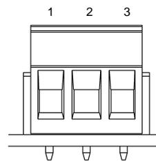
Figure 6 Pluggable Connector on LONWORKS Terminal Block
