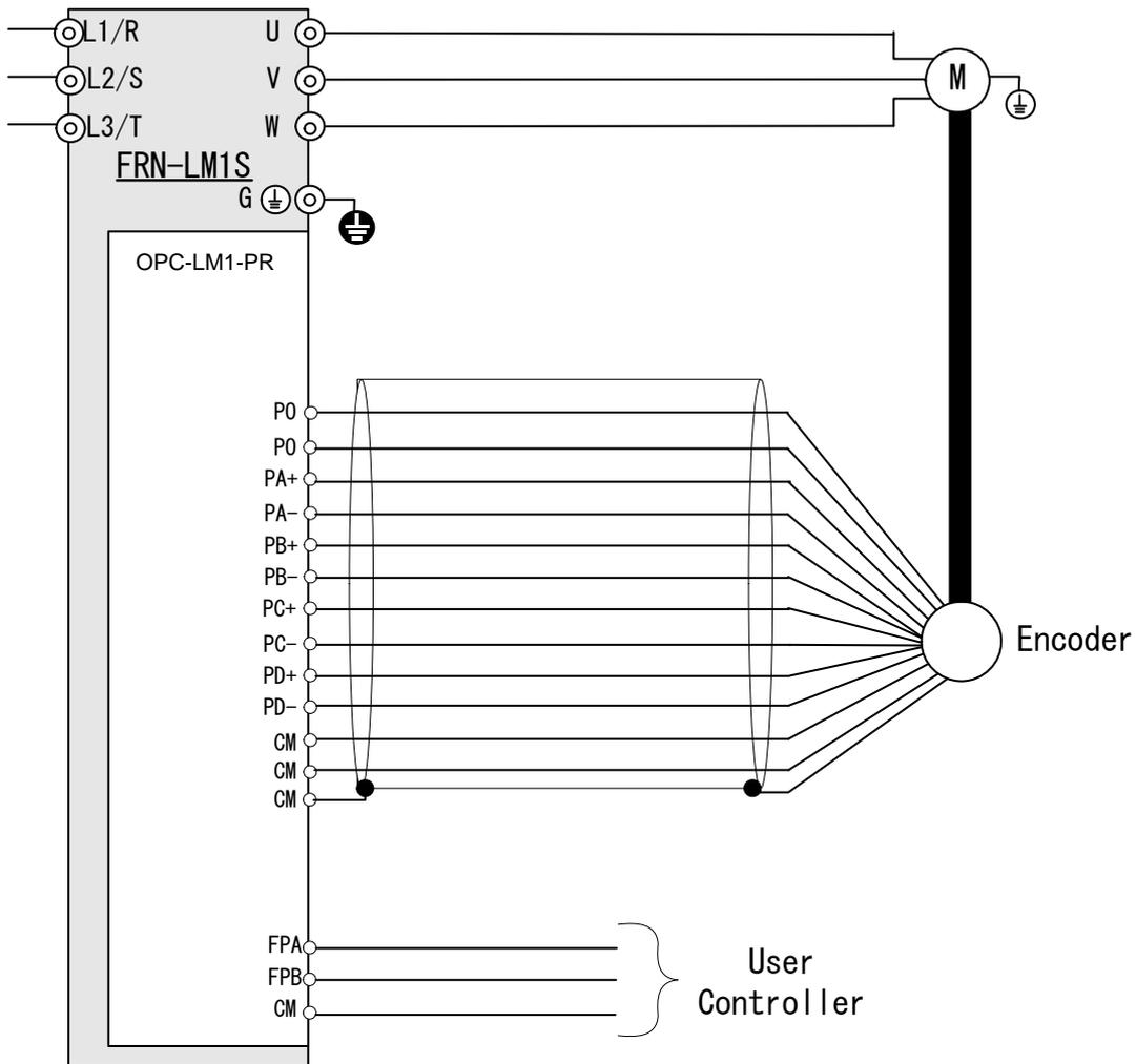
Figure 4.1 Basic Wiring Diagram
