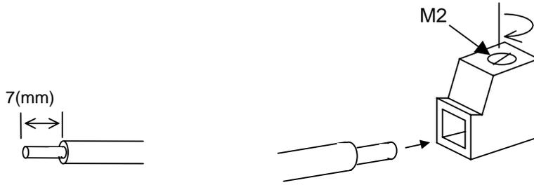
Connection of Wiring on Option Terminal Side.
