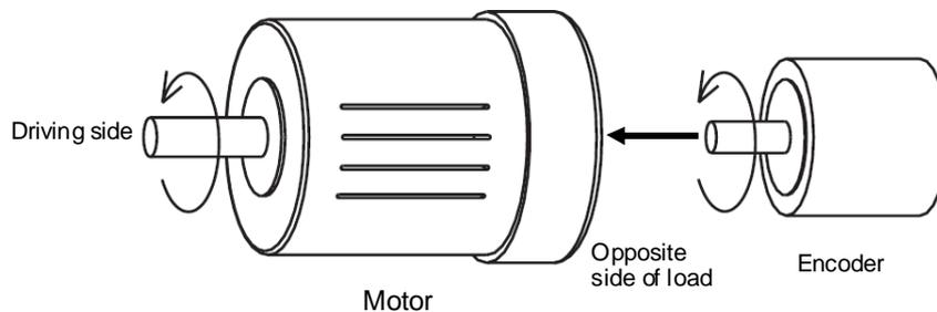
Figure 3.1 Motor and Encoder Rotational Direction when Terminal FWD is ON
