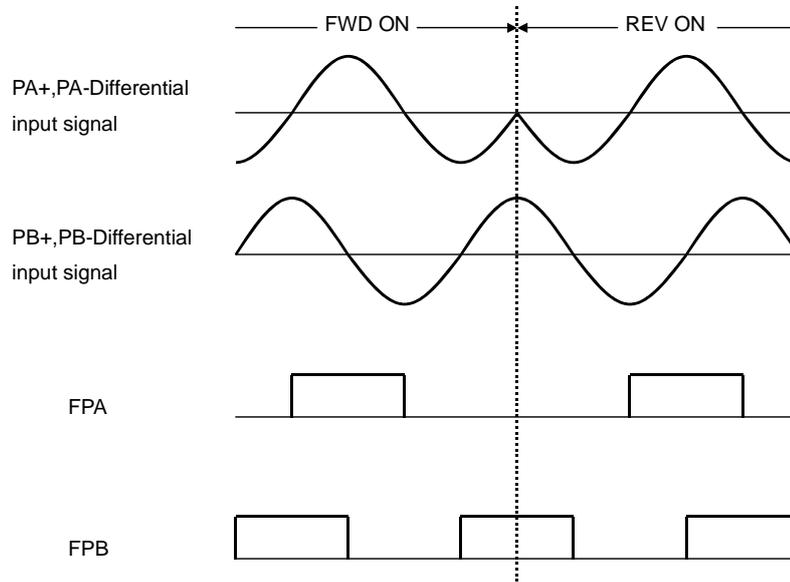
Figure 3.2 Definition of Terminal FWD ON/REV ON
