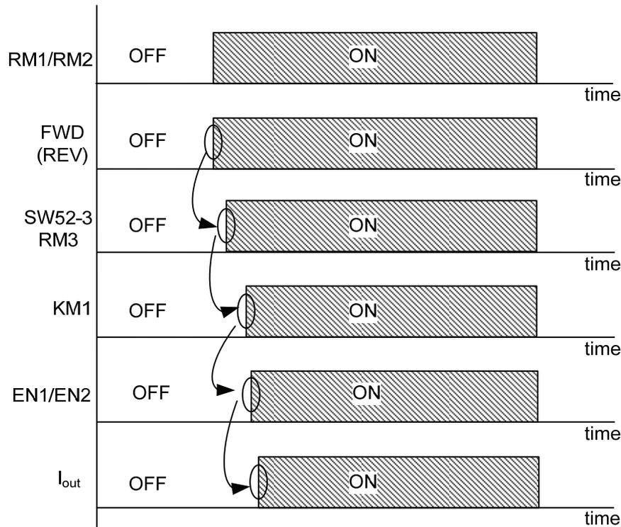
RM1/RM2: Relay for the activation of enable inputs state
