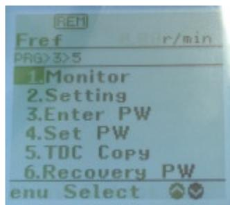
Figure 8. Set password menu to enable TDC function
