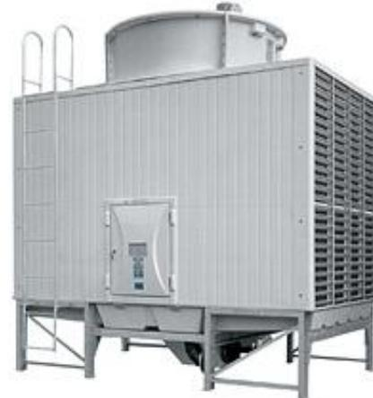
Using Fuji Electric frequency inverters for controlling the speed of cooling tower fan allows keeping the cool water temperature constant thanks to the powerful set of PID functions in the inverter. Great energy savings can be achieved by combining built-in automatic energy savings function and wet-bulb temperature presumption control.
