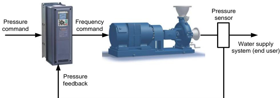
A PID control is a regulation system involving the set value (SV – pressure/flow command) and a process value (PV - Feedback, measure of real pressure or flow from a transducer). From these two values the difference, or error, is calculated, subtracting one from the other. The PID control then adjusts its output demand (MV - pump’s speed) in order to minimize the error.
