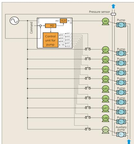
Control of multiple pumps on 1 regulated pump + auxiliary pumps topology (Mono-regulated pump Control)
