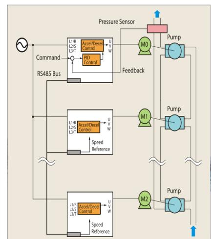
Control of multiple inverters without external controller. Mutual regulated pumps topology (Mutual-regulated pump Control)
