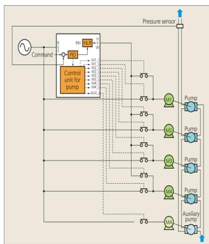
Control of multiple pumps on multi regulated pumps topology (Multi-regulated pump Control)
