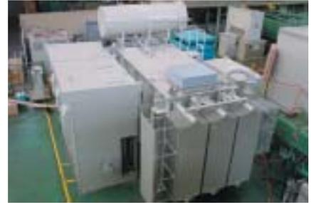
▲ DC power supply for electrolysis (rectifier placed on side)
