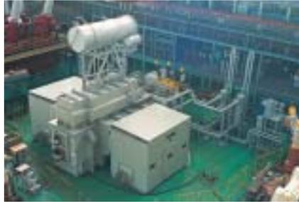
▲ Large-capacity DC power supply for electrolysis (S-Former)
