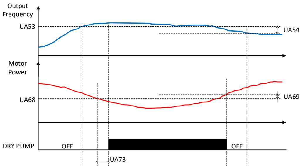
Function code U124 is used to enable the alarm "OH2" in case that dry pump state is detected, by setting this function code to 1.00.
