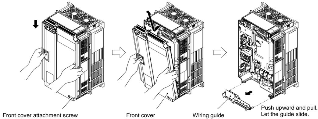
Figure 2.2-3 Removal of the Front Cover and the Wiring Guide (for FRN0072E2-4□)
