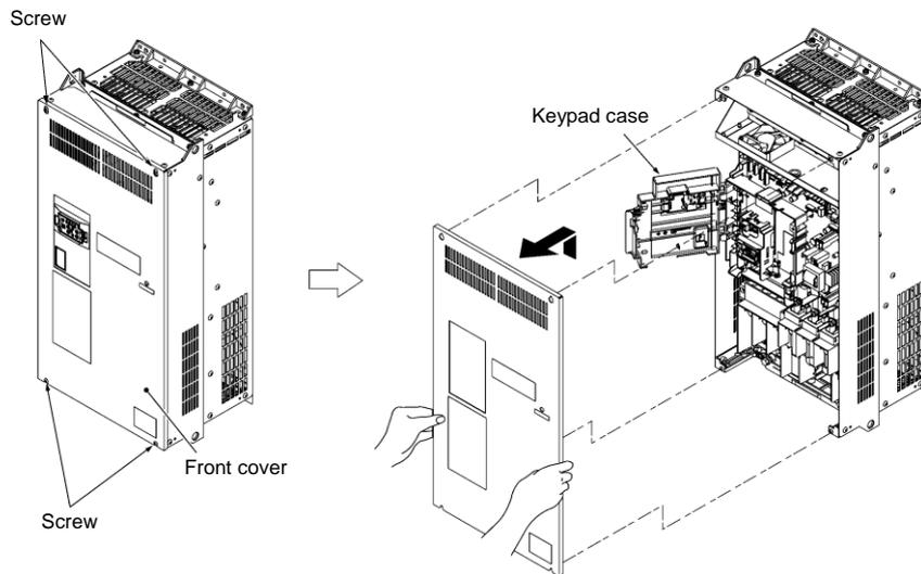
Tightening torque: 1.8 N·m(15.9 lb-in) (M4)
