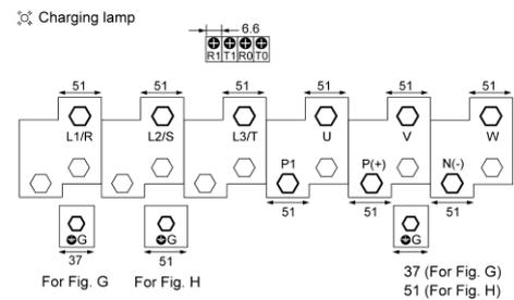
Figure 2.2-7 Main circuit terminals layout
