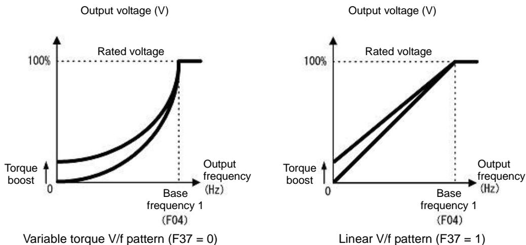
**Tip** When the variable torque V/f pattern is selected (F37 = 0 or 3), the output voltage may be low at a low frequency zone, resulting in insufficient output torque, depending on the characteristics of the motor and load. In such a case, it is recommended to increase the output voltage at the low frequency zone using the non-linear V/f pattern.
