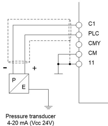
The maximum scale of the pressure transducer can be set in UJ18, parameter. This will scale the meaning of the pressure transducer 4-20mA, as well as the PID setpoint in parameter U122.
