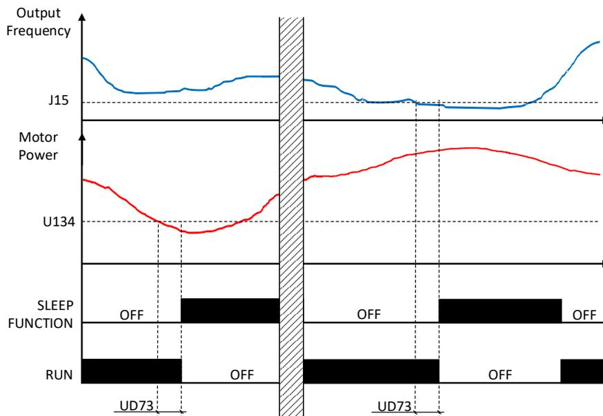
**Note** Do not change the value of function code J17 from factory default value, otherwise it would interfere with the sleep and wake up functions
