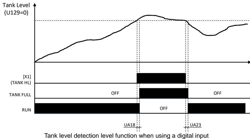
U129 is used in order to invert the function behavior to make a dry pump protection with the analogue input. If U129 = 1, the inverter will stop when the analogue input value is under U128 value and will run again when the analogue input value rises above the U128 + UA14 (applying the corresponding delay times as explained before). U129 default setting is set to 0.
