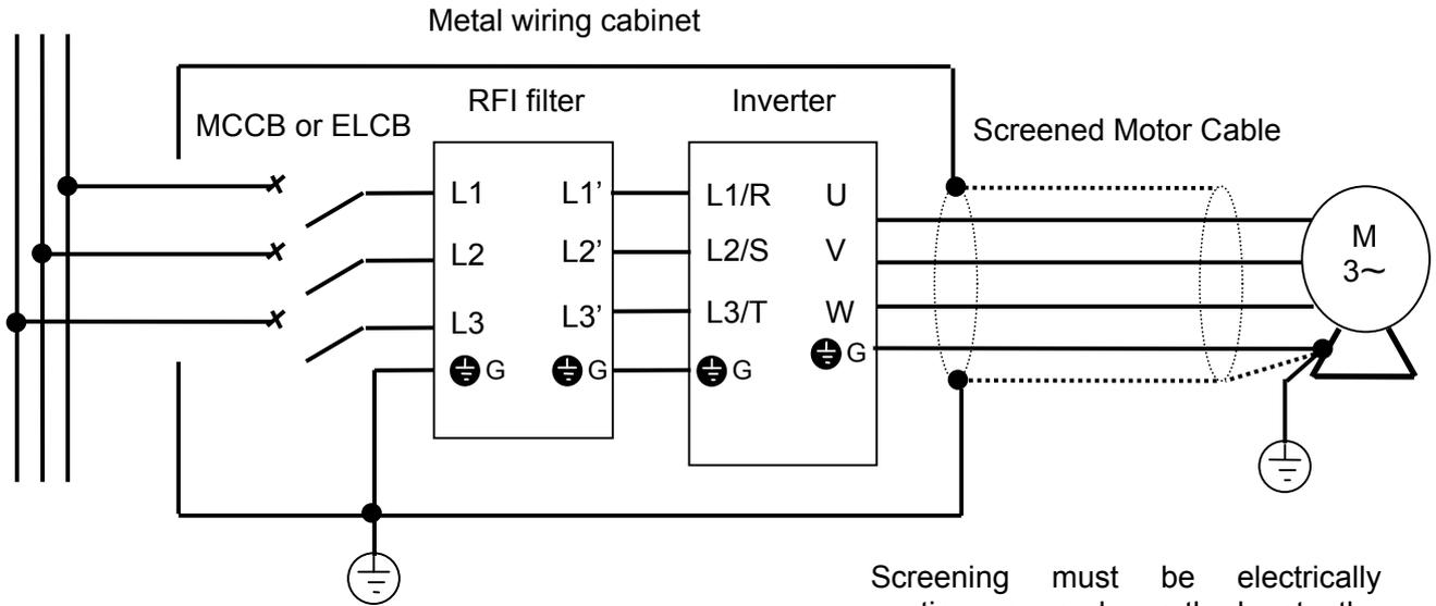
Screening must be electrically continuous and earthed at the cabinet and the motor.
