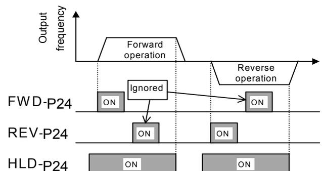
Note : The inverter operates while FWD-P24 or REV-P24 is ON even if HLD-P24 is OFF. An external interlock sequence, which makes FWD-P24 and REV-P24 OFF when HLD-P24 is OFF, is required.
