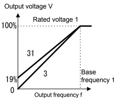
Note) When the torque boost value is excessively large, the motor is excessively excited in the low speed zone at all types of characteristics. If operation continues in such a state, the motor may be overheated. Set a value according to the characteristics of the driven motor.
