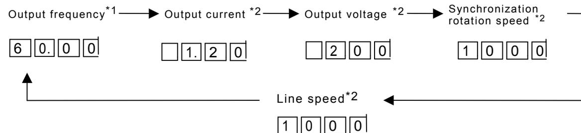
\*1: In the PID control mode (when function H20 is at "1" or "2"), the value is in the percent display and the dot at the least significant digit always lights up.
