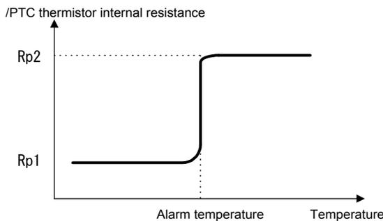
From the figure of H26 "PTC thermistor (Operation selection)", the 250-ohm resistor and the PTC thermistor (resistance Rp) configure a parallel circuit. Therefore voltage VC1 (operation level) of terminal [C1] is calculated in the following equation.
