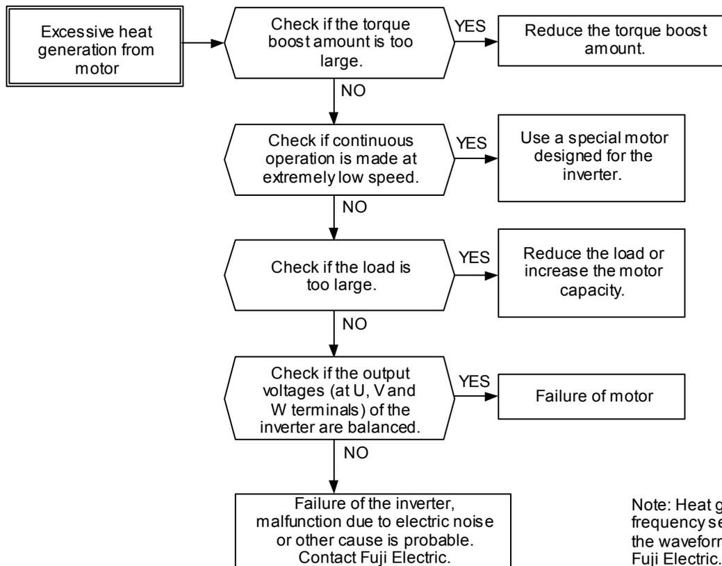
Note: Heat generation with a large frequency setting may be caused by the waveform of the current. Contact Fuji Electric.
