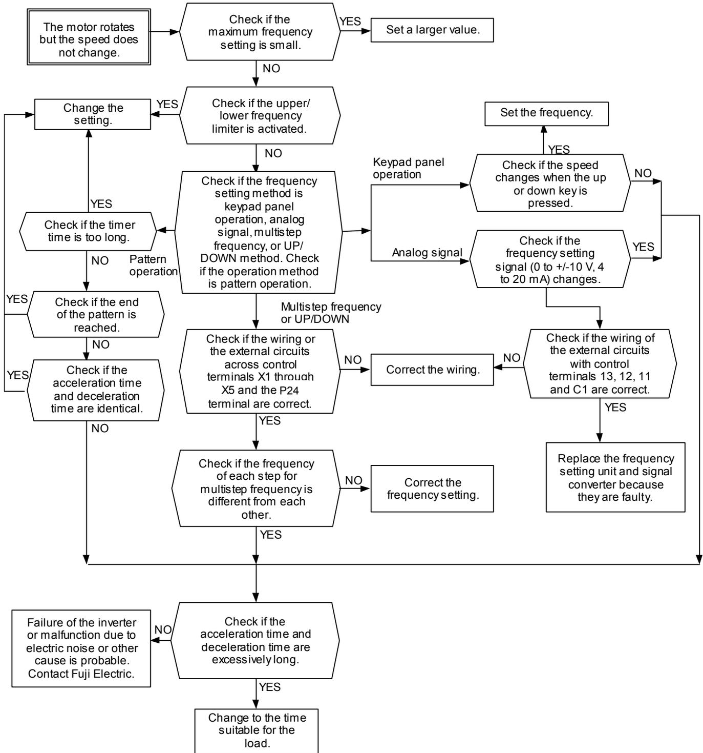
The change in the rotation speed of the motor is also small in the following cases.
