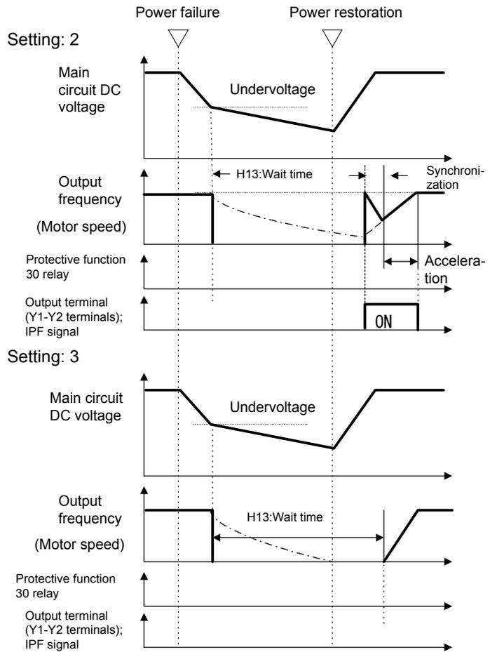
Note: The chain line indicates the motor speed.
