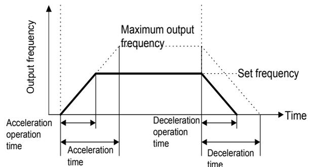
Note) If an excessively short acceleration or deceleration time is set though the load torque or moment of inertia of the load is large, the torque limiter or stall prevention function is activated. When these functions are activated, the time becomes longer than the operation time explained above.
