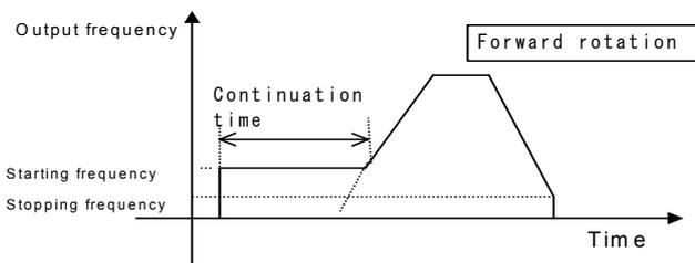
When the starting frequency is smaller than the stop frequency and the frequency setting is smaller than the stop frequency, operation does not start.
