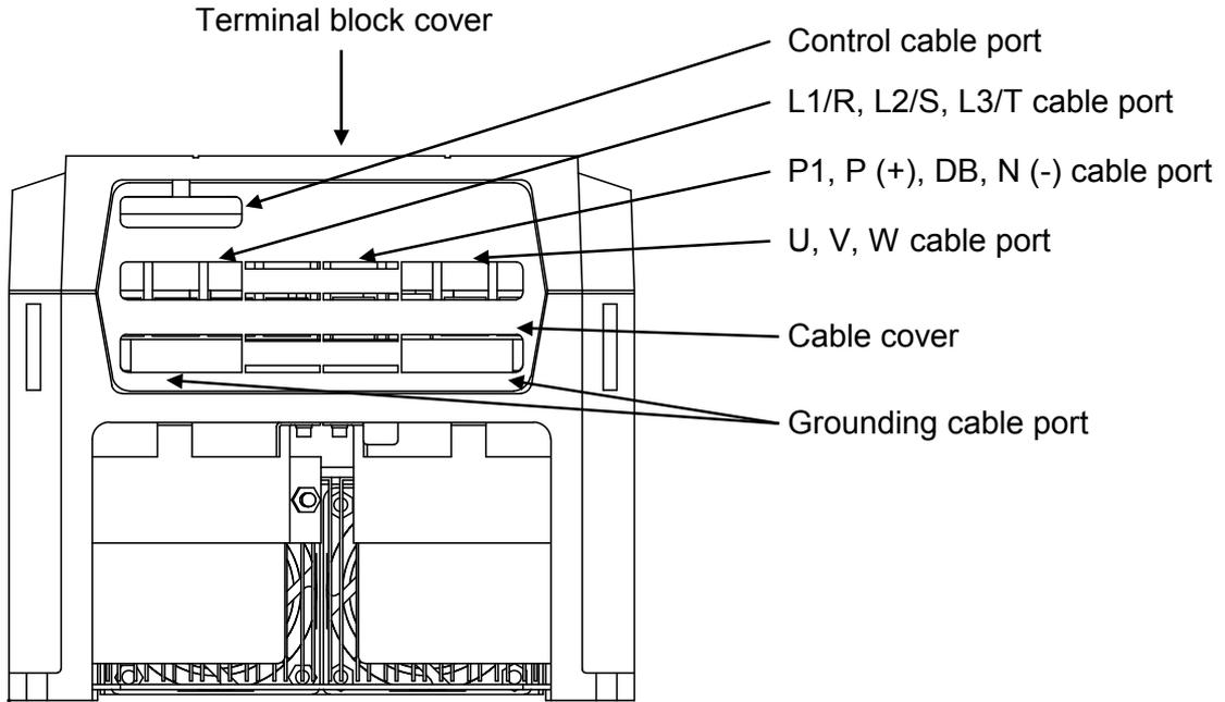
A barrier is provided in the cable cover for the P1, P (+), DB and N (-) cable port. Cut the barrier using nippers or the like before wiring.
