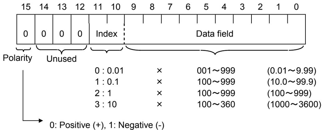
Example: In the case that F07: communication No. (acceleration time 1) = 20.0 seconds
