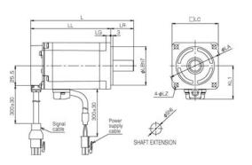
MASS Rated speed Rated output Flange dimensions Model codes L LL S LΖ [r/min] [kW] LR LG LB KL1 LC LA [Kg] GYB201D5-□B2 0.2 112 82 30 6 50 43 60 70 5.5 14 1.0 0.4 3000 GYB401D5-□B2 134 104 30 6 50 43 70 5.5 14 1.5 60 0.75 GYB751D5-□B2 157 117 40 8 70 53 80 90 7 19 3.0
