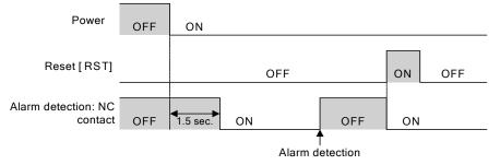
The signal will be off for up to 1.5 seconds after the power is turned on. Check the signal status waiting for 1.5 seconds or more after the power is turned on.
