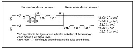
■ Differential input, A/B phase pulse (reference value of parameter 03: 2)
