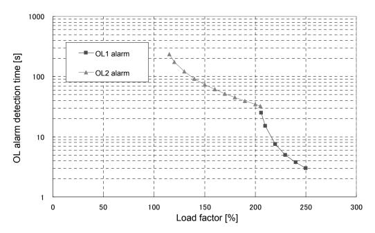
(3) In case of operation at rated rotation speed (2000 r/min) Target capacity: 4.0 kW to 7.0 kW
