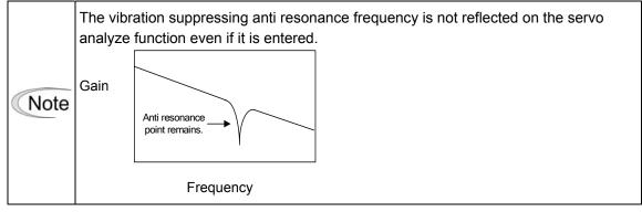
(6) Finely adjusting the vibration suppressing anti resonance frequency While checking effects of vibration suppression, finely adjust the reference value (in increments of 0.1 or 0.2).
