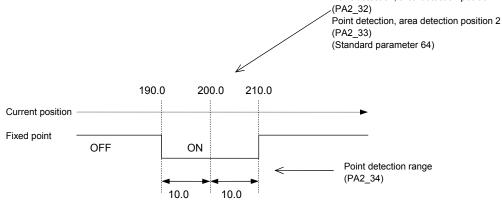
(2) Area OFF  $\rightarrow$  ON (If PA2\_31 (point detection, area detection) is 1)
