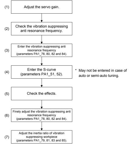
(1) Adjusting the servo gain To ignore the vibration of the tip of the machine and reserve smooth stopping action of the servomotor free from overshoot, refer to the description given in sections 5.1 through 5.5 to adjust the servo gain.
