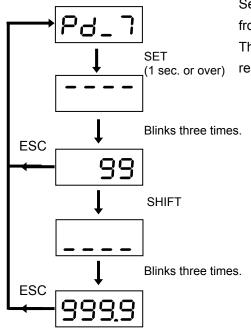
Set the motor deceleration time. The setting value range is from 0.0 to 99999.9 ms in increments of 0.1.
