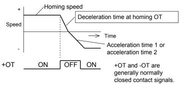
The acceleration time and deceleration time are based on 2000 r/min.
