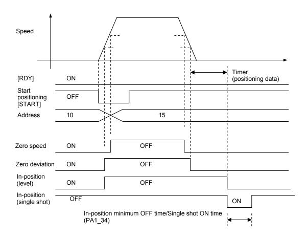
Check for the active state of the in-position signal (level) to turn the start positioning signal on. The motor starts to rotate. After rotation begins, the in-position signal is turned off.
