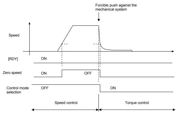
To forcibly push against the mechanical system as shown in the figure above, torque limit should be adopted with a pushing material or the like.
