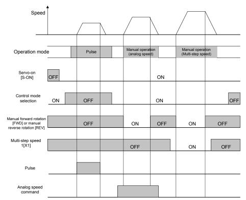
[Example] The operation pattern of control mode selection 3 (position ⇔ speed) is shown in the figure below.
