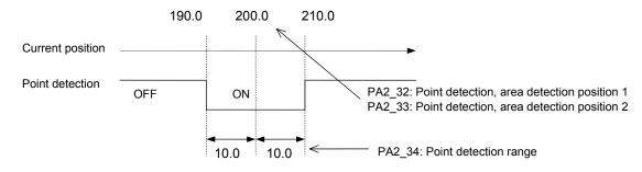
(2) PA2\_31 (point detection, area detection) = 1: ON for positive side
