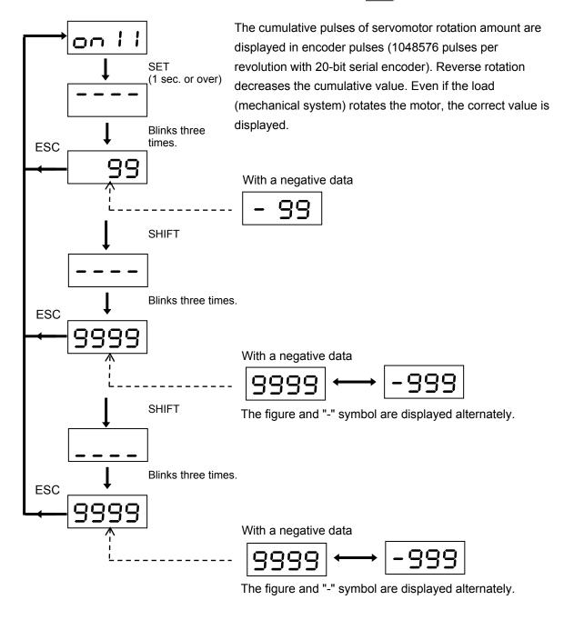
$\begin{array}{|c|c|} \hline \mbox{Hint} & \mbox{Press and hold the } [\wedge] \mbox{ and } [\vee] \mbox{ keys simultaneously for at least one second to reset the feedback cumulative pulses.} \end{array}$
