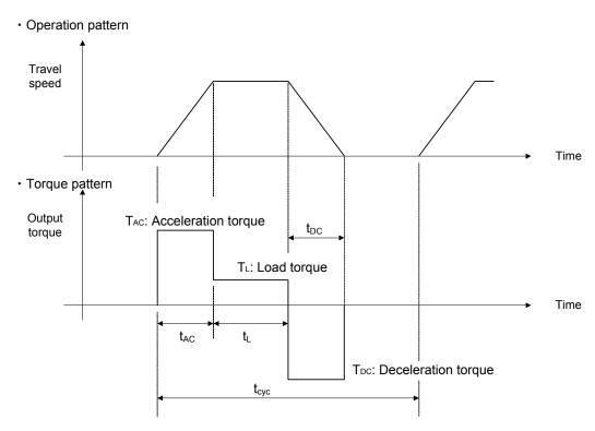
(7) Calculating the effective torque (Trms)Calculate the effective torque of each cycle of the operation pattern.
