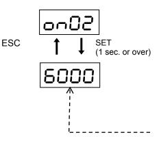
Current speed command issued to the servomotor. The command speed is given in a speed command voltage, multi-step speed, pulse or similar. The speed is displayed in r/min and a negative sign is attached for reverse rotation (clockwise rotation when viewed against the motor shaft).
