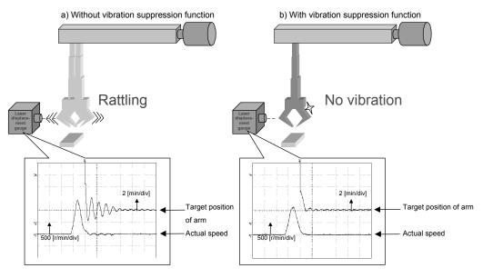
Not only vibration of the tip of the machine but also vibration of the entire machine can be suppressed.
