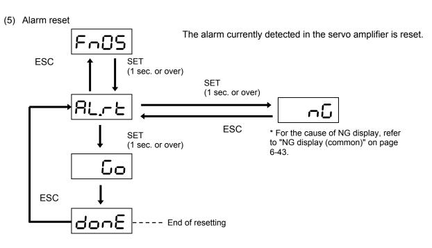
• The servo amplifier is not reset from some alarms through alarm resetting. To reset these alarms, turn the power off then on again.
