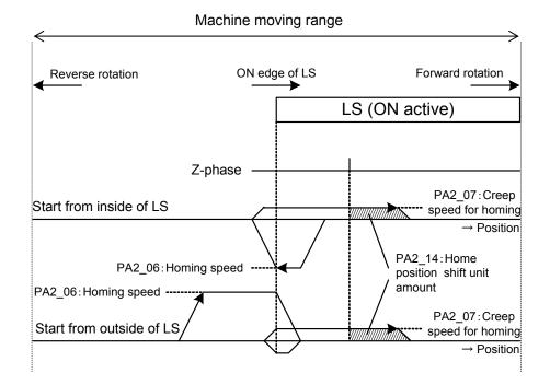
• Operation example at parameter setting change Operation examples after a parameter change necessitated due to the position, etc. of the home position LS (see Table a for the setting example) are shown in Figs. a to c.
