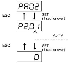
On parameter page 2, parameters related to system setting such as the homing functions are registered. Changes in parameters become enabled after the power is turned off then on again.
