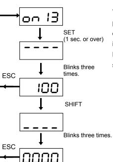
The number of pulses in a homing counted since the home position LS signal is turned off until the Z-phase of the encoder of the servomotor is detected is displayed. The indication is updated every time homing is performed. Because the value is in the homing direction, no negative sign is attached.
