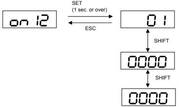
The display example for 10000000-pulse is shown.
