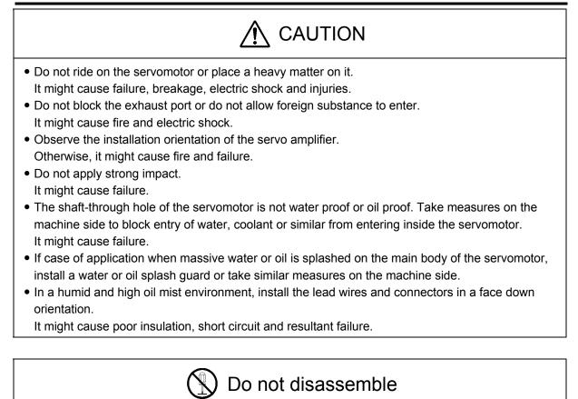
• Never remodel the servomotor and servo amplifier. It might cause fire and failure. It will not be covered by the warranty.
