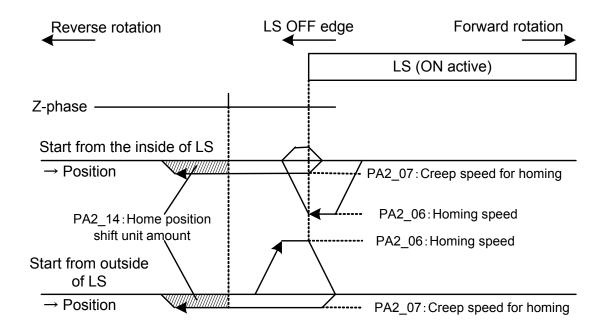
(7) Homing pattern using the encoder Z-phase as a reference signal for homing When it is a machine which cannot install sensors, such as LS, PA2\_12: Reference signal for homing set as "Encoder Z-Phase".
