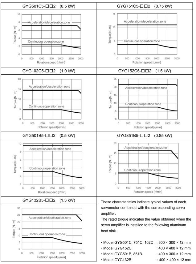
Torque characteristics diagram (at 3-phase 200 V amplifier source voltage)
