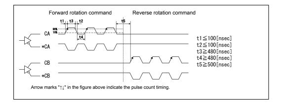
■ Open collector input, forward/reverse pulse (reference value of parameter 03: 11)
