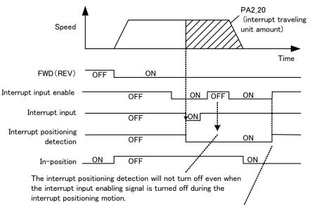
The interrupt positioning detection will turn off if the interrupt input enabling signal is turned off after the interrupt positioning completion ( in-position = ON).
