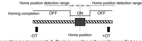
The zero position is not necessarily 0. The home position is the position specified as a home position after homing completion (PA2\_16) or preset position (PA2\_19).
