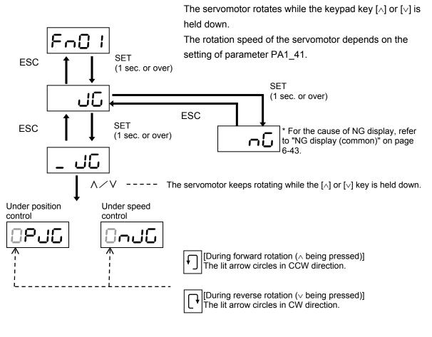
Note The forced stop, external regenerative resistor overheat, ±OT and free-run signals are enabled even during test operation. Check these signals if test operation does not start.
