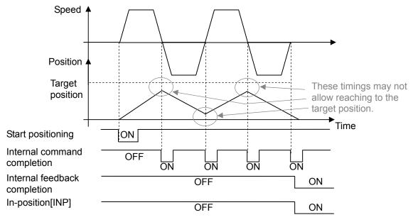
Setting value: 1 (Internal feedback completion.)
