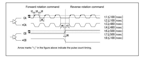
Open collector input, command pulse/direction (reference value of parameter 03: 10)
