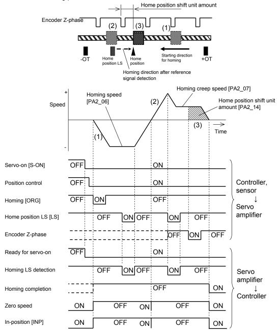
• At the rotation direction selection point with zero speed, zero speed and in-position [INP] are momentarily turned on. The signal change may fail to be sensed according to some scanning periods of the host controller.
