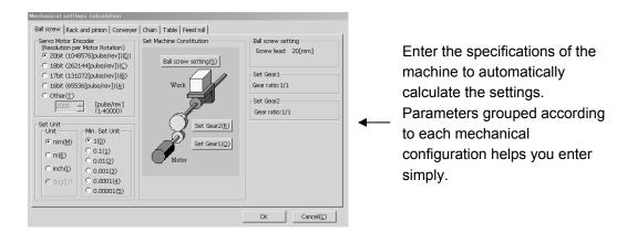
[Example of calculation of electronic gear ratio]
