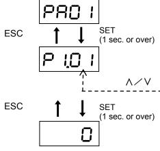
On parameter page 1, relatively frequently used parameters are registered. Changes in most parameters are reflected on the servo amplifier and servomotor operation immediately.
