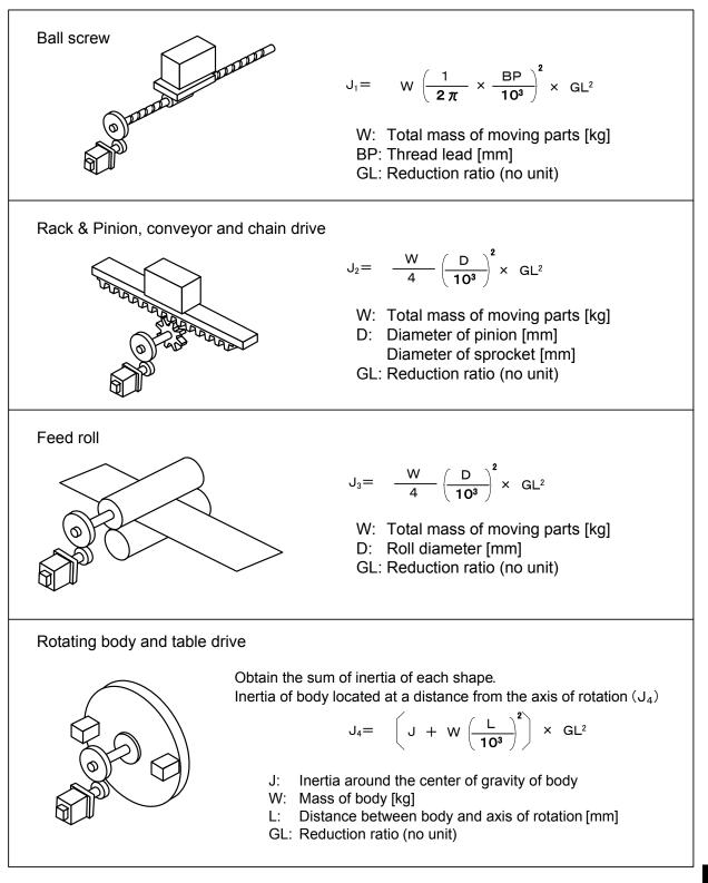
■ Calculation of load torque (TL)
