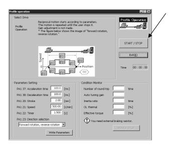
Press the "START/STOP" button to start profile operation. Press the "START/STOP" button during the motion to stop after the current cycle.
