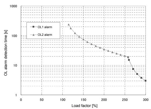
In case of operation at rated rotation speed (2000 r/min) Target capacity: 1.0 kW to 3.0 kW
