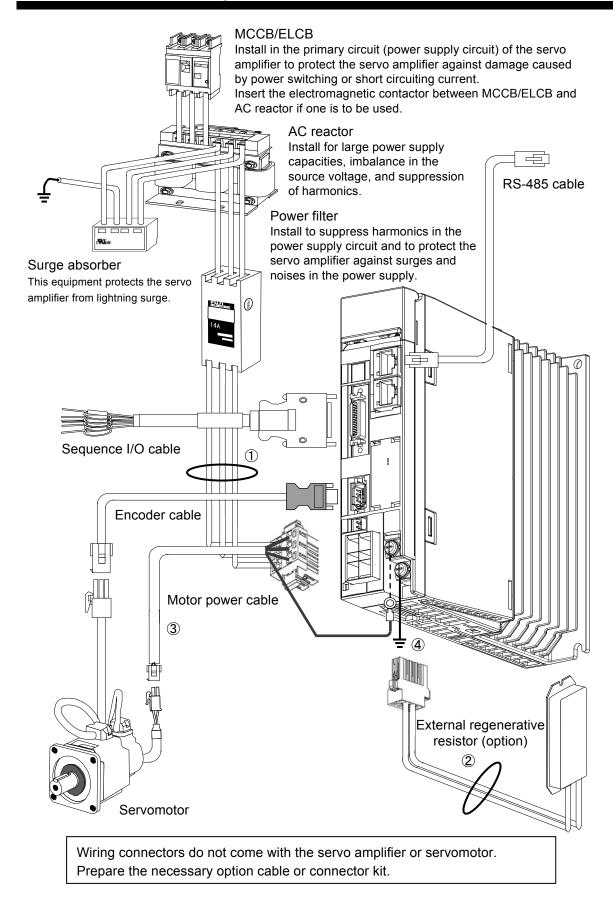
10-2 Overall Configuration of Peripheral Equipment
