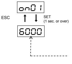
Current rotation speed of servomotor.
