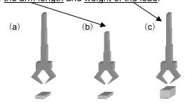
The vibration suppressing anti resonance frequency varies according to conditions a, b and c.
