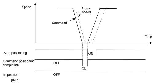
If a motion to the current position is started, the servomotor does not start but the in-position signal is turned off for the time specified in PA1 34 (in-position minimum OFF time / single shot ON time).
