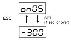
Peak torque value of the servomotor at every two seconds; the torque is displayed in percent to the rated torque. The range from 0% to the maximum torque is displayed in increments of 1. In case of a negative peak torque, a negative sign is attached to the most significant digit. (6) Effective torque (displayed digits: signed three digits)
