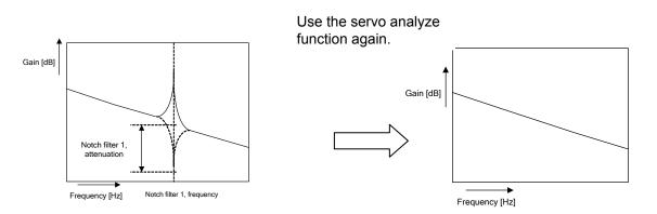
The notch filter is added to the resonance point as shown in the figure above.
