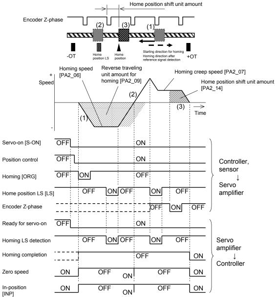
• At the direction of rotation switch rotation direction selection point with zero speed, zero speed and in-position [INP] are momentarily turned on. The signal change may fail to be sensed according to some scanning periods of the host controller.
