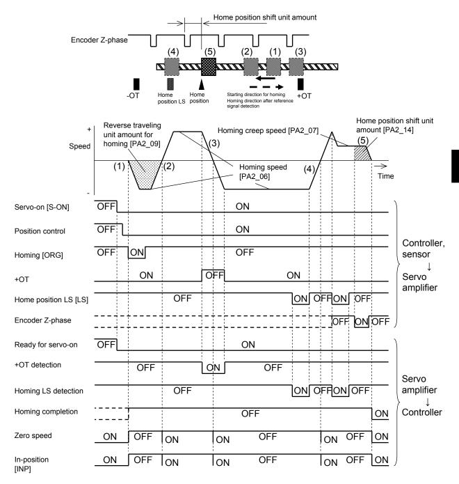
(4) Reference signal for shift operation homing profile (equivalent to homing profile 4 of FALDIC- $\alpha$  Series)
