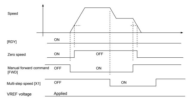
Use parameter PA3\_35 to specify the zero clamp level in relation to the [VREF] input.
