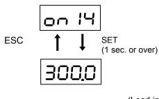
The load inertia ratio recognized by the servo amplifier without relations to parameter PA1\_13 (tuning mode selection) is displayed. The value is displayed in a multiple (in 0.1 increments) to the inertia of the servomotor itself. The displaying range is from 0.0 to 300.0 times.
