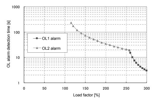
(1) In case of operation at rated rotation speed (1500/2000 r/min)
