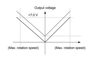
Specify the negative sign for the monitor 1/2 scale to reverse the polarity of the output voltage.
