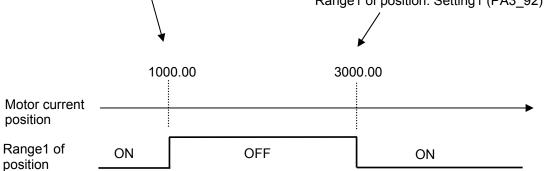
Note: If setting 1 of range 1 of position (PA3\_92) is the same as setting 2 of range 1 of position (PA2\_93), range 1 of position is always turned off. The same is true for range 2 of position.
