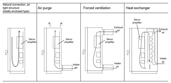
(3) To install two or more servo amplifiers in the same control panel, the following shall be taken into consideration.
