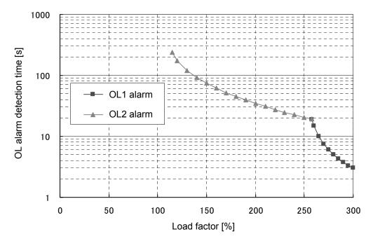
(2) In case of operation at maximum rotation speed (6000 r/min) Target capacity: 0.05 kW to 0.75 kW\*
