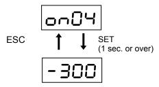
Current flowing through the servomotor; the current is displayed in percent to the rated current. The range from 0% to the maximum current is displayed in increments of 1. In case of a negative motor current, a negative sign is attached to the most significant digit.
