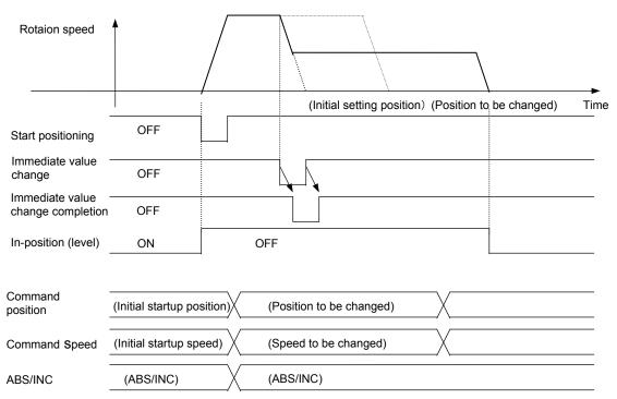
The command position and command speed change at the rising edge of the immediate value change command. They can be changed at an arbitrary timing while the in-position signal remains inactive.
