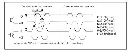
Open collector input, A/B phase pulse (reference value of parameter 03: 12)
