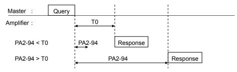
After the master has sent a query, if it takes a long time until the master switches into the receiving state, set PA2\_94 (response time) as needed because responses from the amplifiers might not be received correctly.
