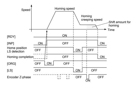
For details of the homing pattern settings, refer to "CHAPTER 4 PARAMETER." The homing motion can be interrupted with forced stop [EMG].
