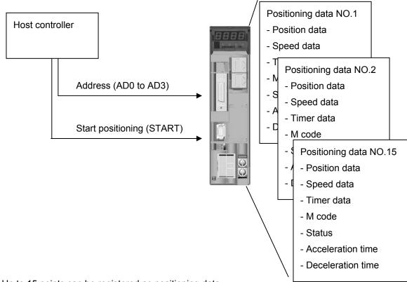
Up to 15 points can be registered as positioning data. Register data, using PC Loader or at the keypad. (2) Immediate value data operation
