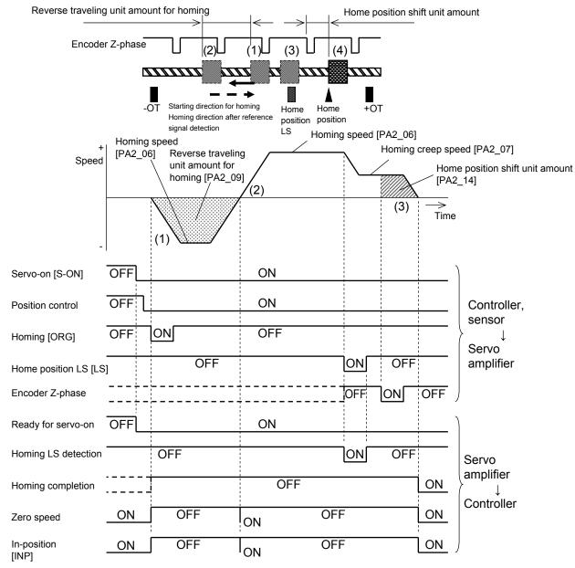
• At the rotation direction selection point with zero speed, zero speed and in-position [INP] are momentarily turned on. The signal change may fail to be sensed according to some scanning periods of the host controller.
