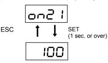
The load ratio to the load alarm level is displayed in percent. An overload alarm is caused if this value reaches 100. The minimum increment is 1. The displaying range is from 0 to 100%.
