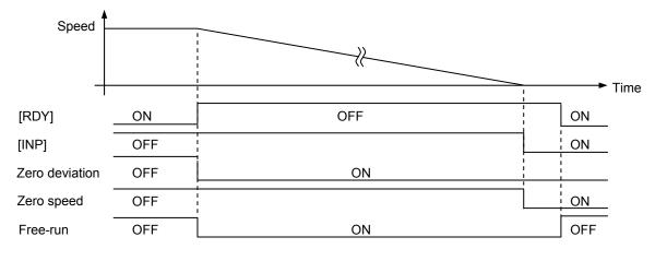
Note In regular cases, free-run is not used for vertical traveling machines. If the function is used for a vertical traveling machine, examine adaptability with the brake carefully.
